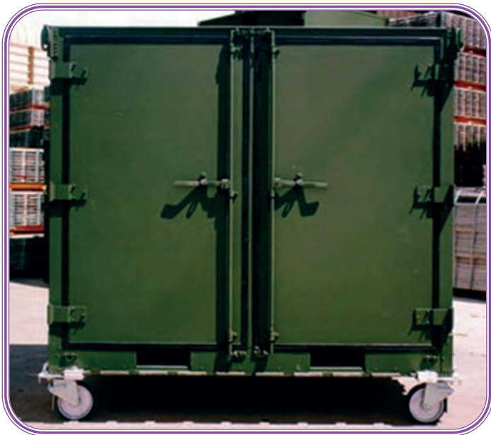
An ISU-90 container. The SORT was designed so that all its equipment could be loaded into three of these units for shipment on Air Force cargo aircraft.
